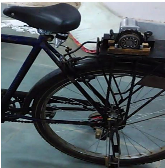
The driving mechanism in the autonomous bicycle
